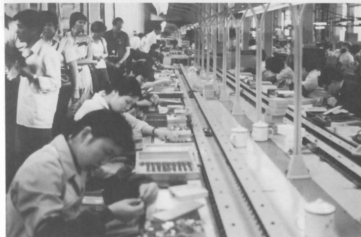
HP visitors (left) view assembly line in Shanghai Electronics Factory #3. Parts and assemblies move by belt.
